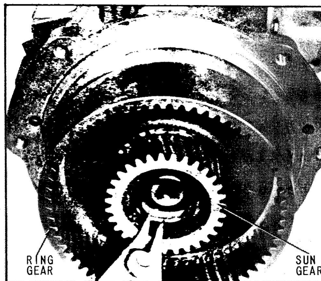
Fig. 25 Remove Snap Ring (3 to 1 Ratio)
