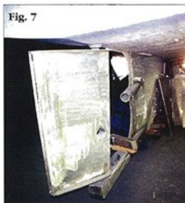
Figure 7 —The Gerr-designed, single-screw motoryacht Imagine is fitted with a MacLear Thistle rudder. Note the endplates top and bottom.
