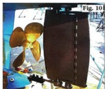
Figure 9 —Articulated flap rudders first appeared in the 1890s. A modern example is this unit manufactured by Deflector Marine, viewed from the side, turned hard to starboard. Figure 10 —The Deflector rudder on centerline, viewed from astern. Operation of the flap is automatic. Figure 11 —This drawing shows range of motion—45° for the main rudder, 90° for the flap.
