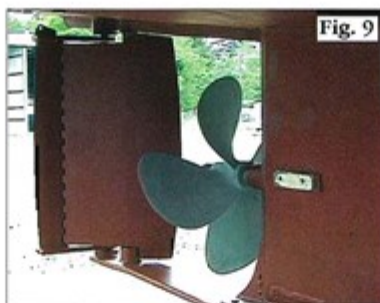
Figure 9 —Articulated flap rudders first appeared in the 1890s. A modern example is this unit manufactured by Deflector Marine, viewed from the side, turned hard to starboard. Figure 10 —The Deflector rudder on centerline, viewed from astern. Operation of the flap is automatic. Figure 11 —This drawing shows range of motion—45° for the main rudder, 90° for the flap.
