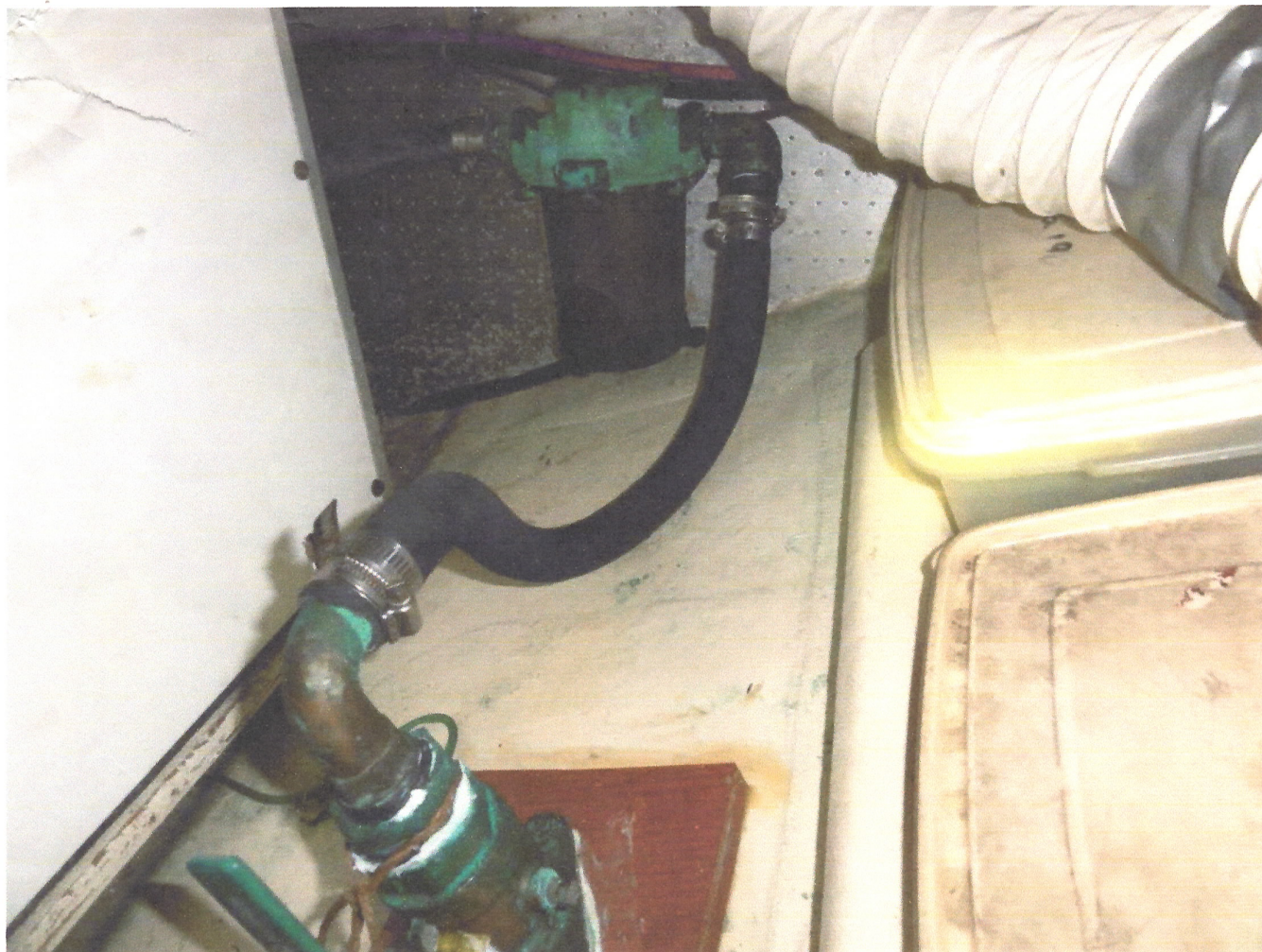
Hose position from through-hull to strainer
