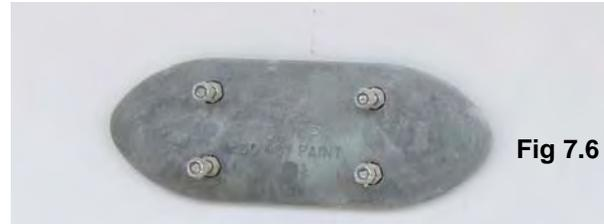
The sacrificial zinc anodes are considerably easier and cheaper to replace and their deterioration will not affect the performance of your boat as would the deterioration of any underwater components.
