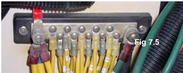
While there are bonding blocks as well aboard your boat, the grounding blocks can be determined by the groups of yellow (negative) wires attached. All electrical circuits require a ground, so all grounds are joined in sections at "grounding blocks".
