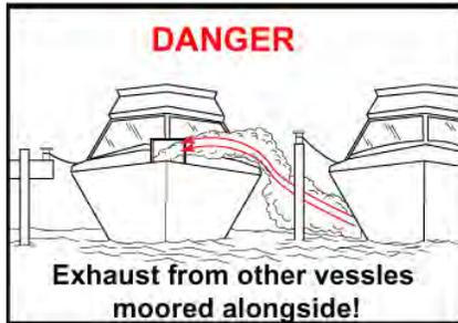
**Figure 4.4.** Engine and generator exhaust from other vessels alongside your boat, while docked or anchored, can cause excessive accumulation of Carbon Monoxide gas within the cabin and cockpit areas of your boat. Be alert for exhaust from other vessels.
