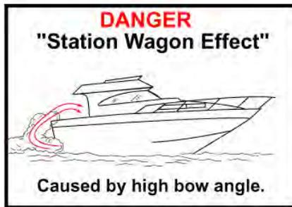
**Figure 4.5.** Engine or generator exhaust from your boat while underway and operating with a high bow angle can cause excessive accumulation of Carbon Monoxide gas within the cabin and cockpit areas of your boat. Always provide adequate ventilation and redistribute the load to lower the boat angle.
