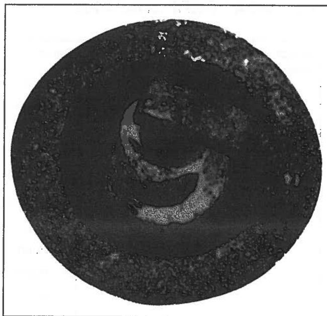
Figure 5-10. Deposit-Damaged Plug
