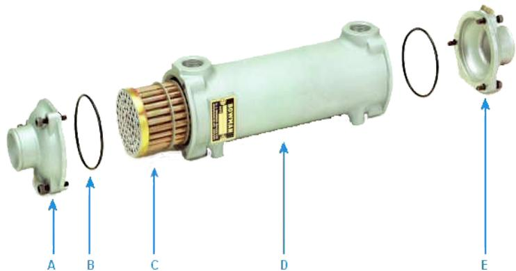
Take a look at the pic of a disassembled heat exchanger. You can usually remove the end caps (A and E) and pull the core (C) from the shell (D) for cleaning. When you reassemble, use new gaskets (B) and lots of waterproof grease to limit corrosion.
