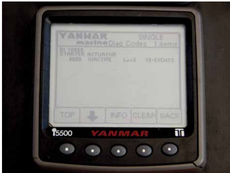
The digital instrument panel at the helm gives you access to error codes and a direct route to problem solving the issue.
