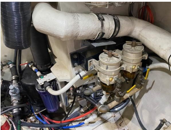
In-line filters/ fuel polisher system detail. (there are 7 in-line fuel filters plus mounted engine filters).
