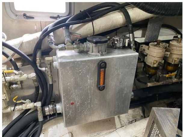
Hydraulic oil tank for stabilisers. The second hydraulic oil tank is below the red tool box in the next picture.
