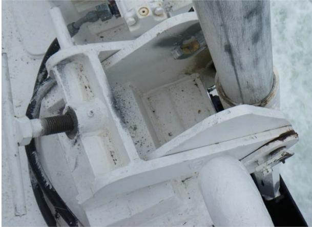
Guide rail: Holds and guides the sliding arms when the fins are deployed. A retaining pin is recessed in the bottom of the rail to hold the sliding arm in place.
