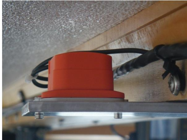
A. Inertial motion sensor, attached to the ceiling of the wheelhouse in each of the two crabbers
