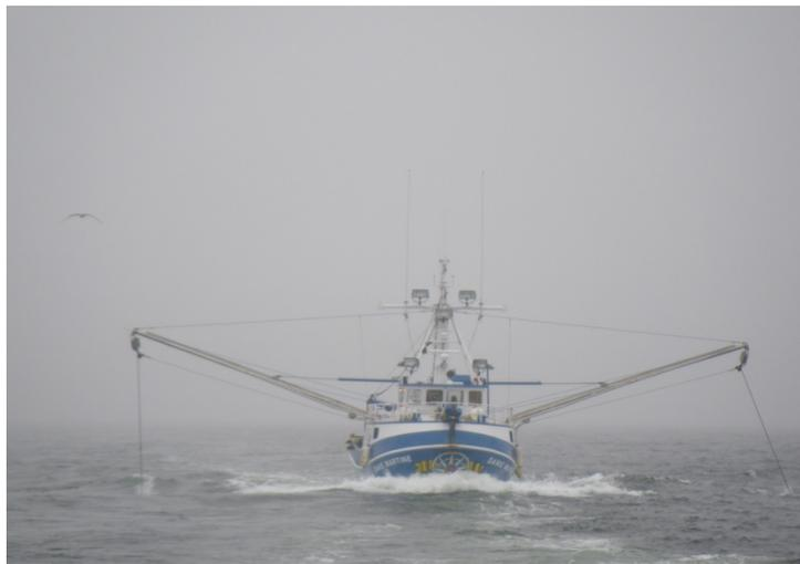
**Figure 1. Paravane roll-damping system**
