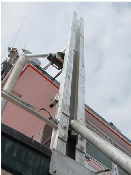
Latch: This is a moving part attached to the fixed bar linkage, it snaps back against the end of the sliding arm to hold it in place when the fin is deployed.
