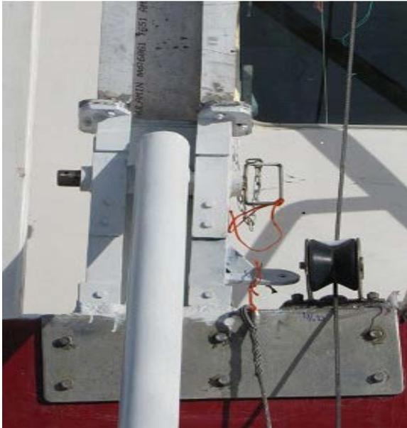
Sliding arm: Rod that keeps the fin immersed at a given angle and depth so that it will fulfil its function.
