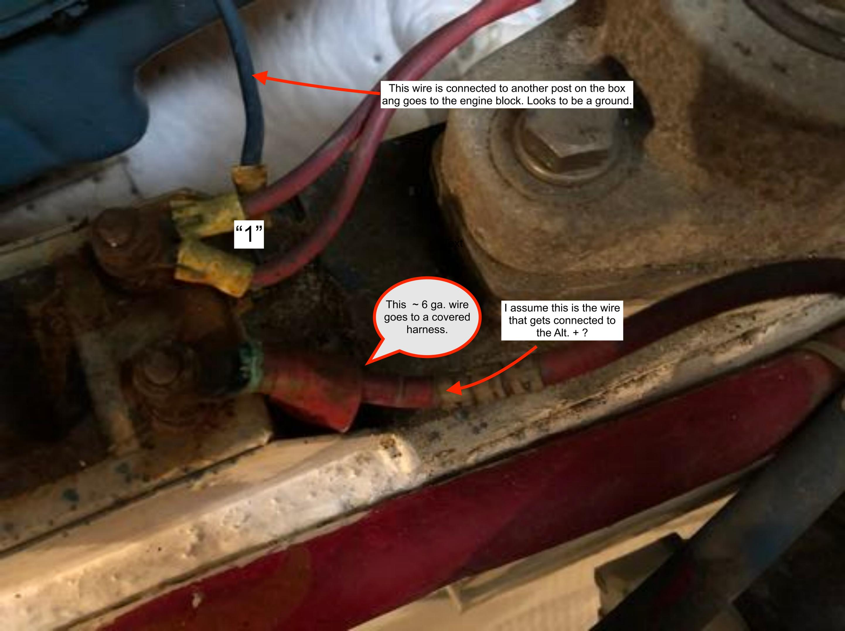
This wire is connected to another post on the box and goes to the engine block. Looks to be a ground.
