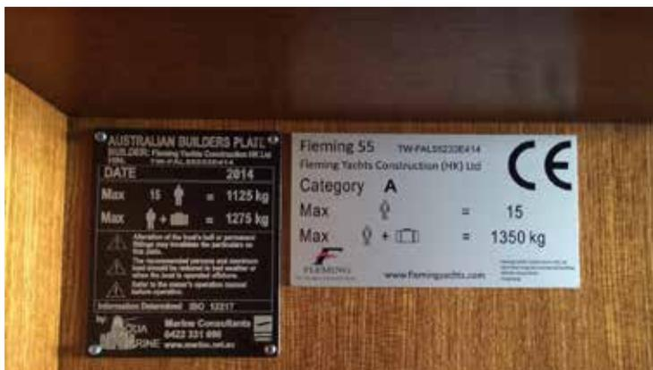
*Depending upon the region for which a Fleming is built, it may be required to display builder's plates like those shown here, certifying in this case that the vessel meets both Australian and CE construction standards.*
