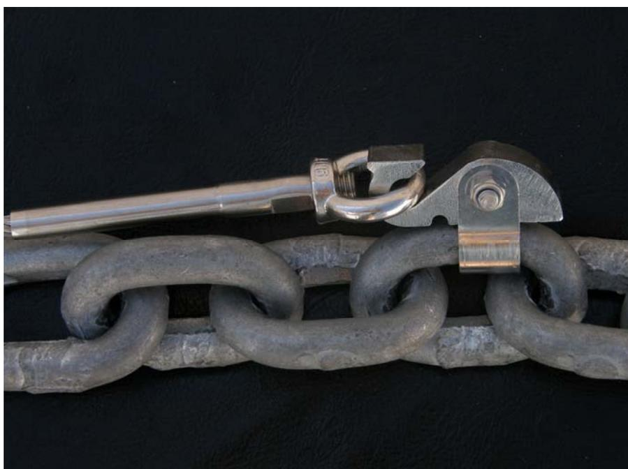
7. All that is left now is to close the holder with a length of the 0,5 mm wire tied with a few turns with the help of a pair of pliers as shown. This closing wire will be replaced after every use of the **AnchorWitch**.
