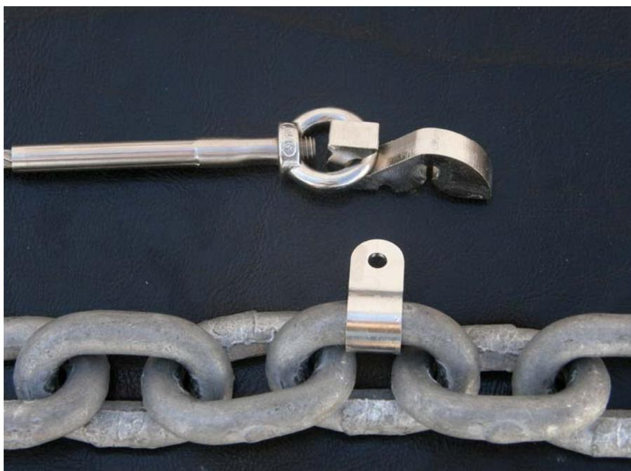
**6.** Now let us pass the bolt through the shackle and the hook and tighten the nut.
