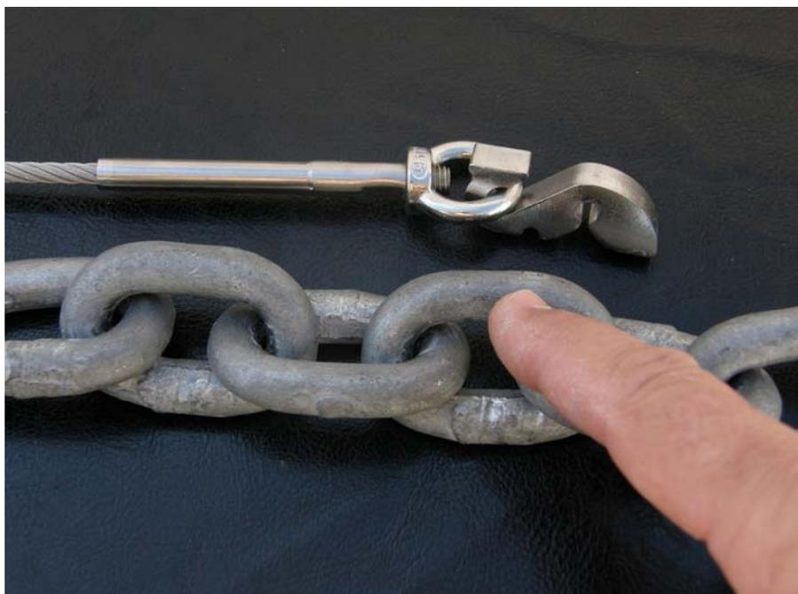
**5.** It is time to mount the wire holder on the selected link. To enable unrestricted movement, it is better to pass the shackle on the smooth side of the link, not on the welded one. If necessary we can turn the chain upside down to have the smoother part on the upper side.
