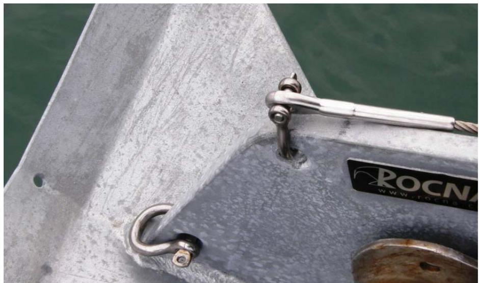
**4.** When selecting the chain link for attaching the wire holder, choose the first vertical link to which the wire strop can be connected without being taut when the chain is pulled, as in the photograph, since there is no need for additional slackness. When the anchor is parked on the roller, vertical links are normally on the same plane as the anchor's shank, and we select one of these so that the wire holder is always facing the anchor when submerged.
