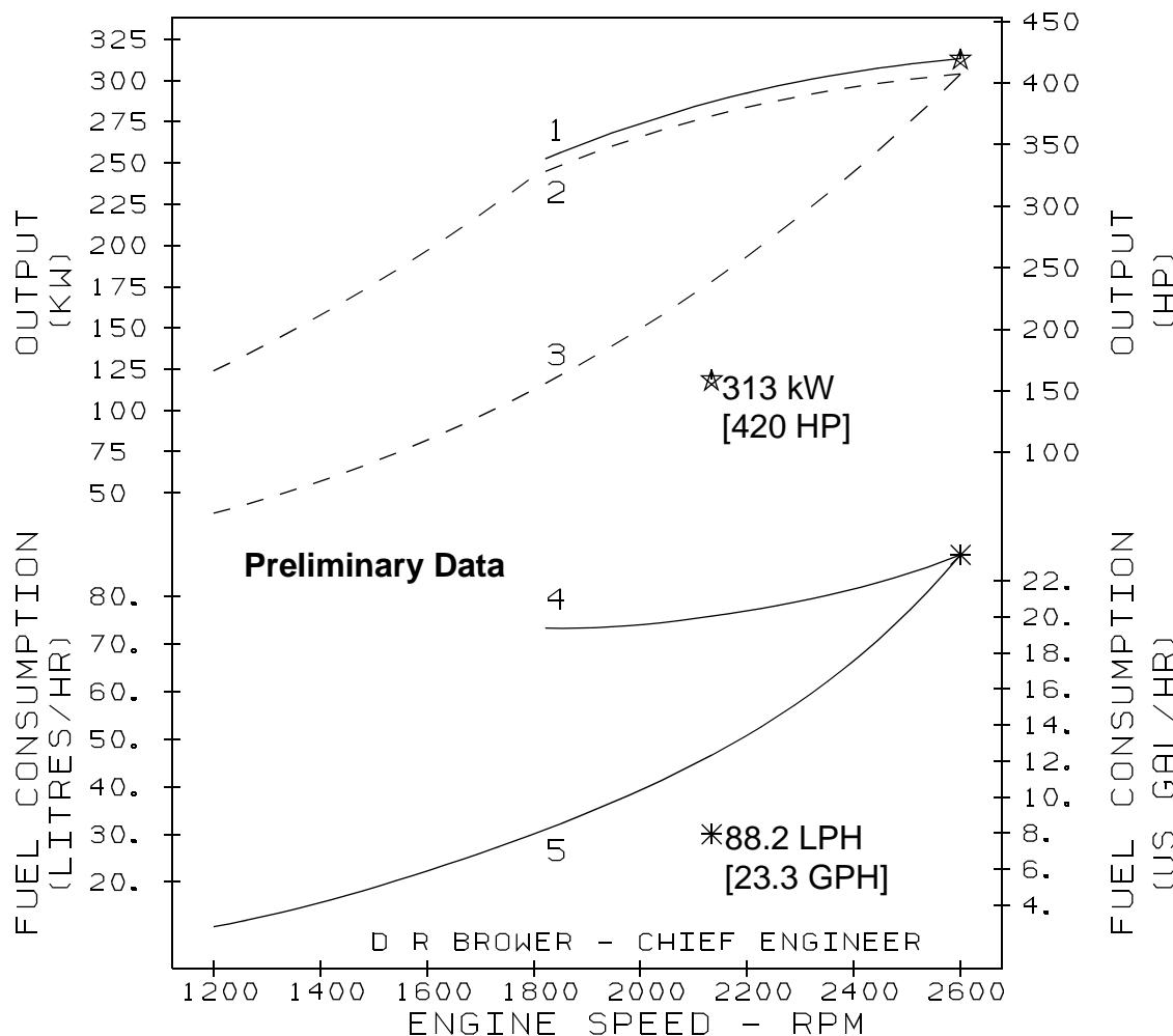
Rating Conditions: Ratings are based upon ISO 8665 conditions of 100 kPa [29.612 in. Hg] 27°C [81°F] and 60% relative humidity. Propeller Shaft Power represents the net power available after typical reverse/reduction gear losses and is 97% of rated power. Fuel consumption is based upon No.2 diesel fuel with a fuel weight of 0.85 kg/litre [7.1 lbs per U.S. gal] and the power requirements of a typical fixed pitch propeller. Power rated in accordance with IMCI procedure.
